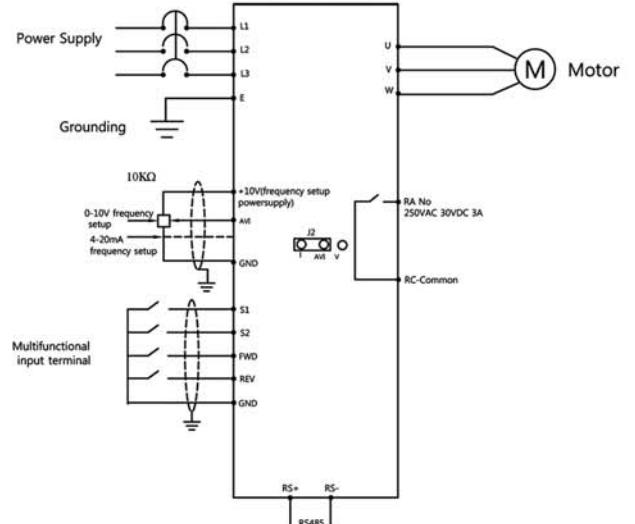
Note:AVI terminals can be used to select an analog voltage input (0-10V) and current input (4-20mA) through the switch J2
